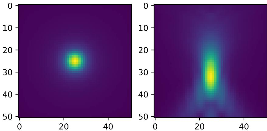
Note how much worse the axial performance is from the spherical aberration induced by RI-mismatch between the sample and immersion oil!
